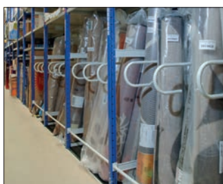
Vertical Storage - Stores long thin items on their ends for better space utilisation within a shelving bay.
