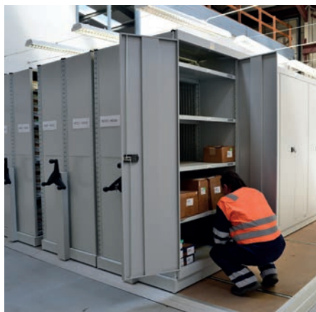
Using pin hinge doors allows cupboards to be created within shelving runs to offer secure storage for valuable items.
